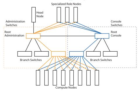
Figure 3-3 shows a graphical representation of the logical layout of the switches and nodes in a large-scale system with a Super Root Switch. The head node connects to Port 42 on the Root Administration Switch in Region 1.
